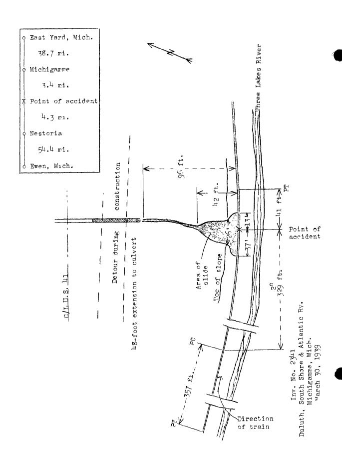
The track structure at the point of accident consists of 80-pound rail, 33 feet in length, laid on 19 hemlock ties to the rail length; it is double-spiked on the inside and single-spiked on the outside, fully tieplated, ballasted with 10 to 12 inches of gravel with 10 inches of stamp sand below the tops of the ties, and is fairly well maintained.
